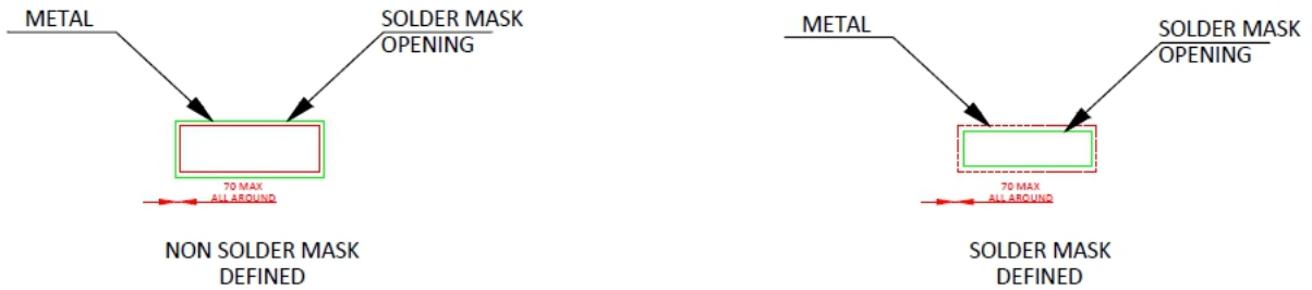
Figure 9.2 SOW8 Package Board Layout Example
