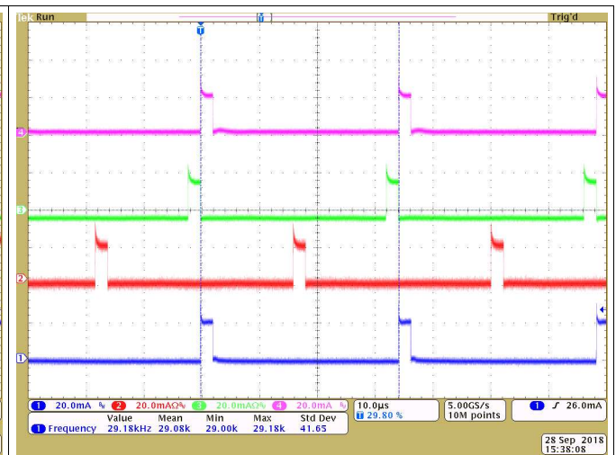
图 63. Current Waveform of OUT0, OUT1, OUT2 and OUT3
