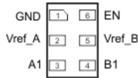
图 5-1. LSF0101 DRY Package, 6-Pin SON (Transparent Top View)
