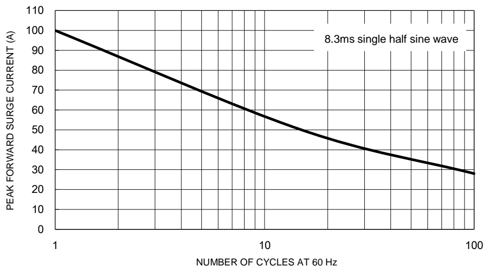
Fig.5 Maximum Non-Repetitive Forward Surge Current
