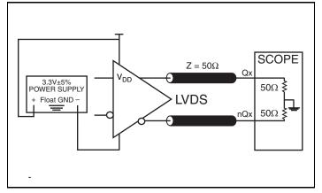
3.3V LVDS Output Load AC Test Circuit
