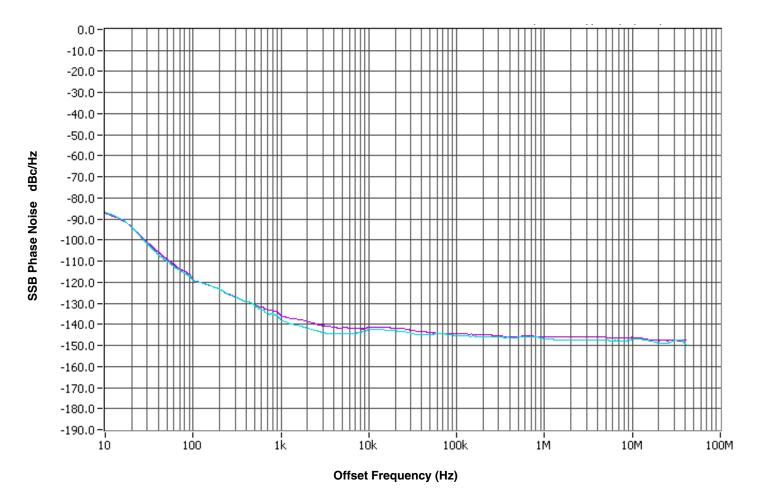
As with most timing specifications, phase noise measurements have issues. The primary issue relates to the limitations of the equipment. Often the noise floor of the equipment is higher than the noise floor of the device. This is illustrated above. The device meets the noise floor of what is shown, but can actually be lower. The phase noise is dependant on the input source and measurement equipment.
