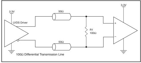
Figure 2. Typical LVDS Driver Termination
