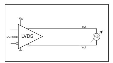
**Differential Output Short Circuit Setup**
