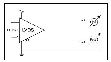
**Output Short Circuit Current Setup**
