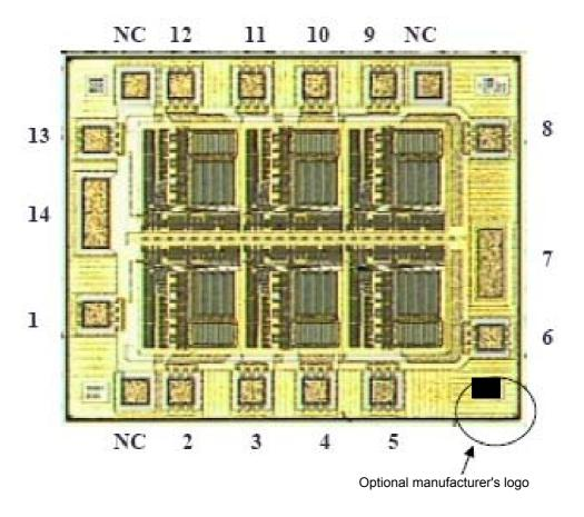
Pad size: Pad numbers 1 to 6 and 8 to 13: 100 x 100  $\mu$ m Pad numbers 7 (GND) and 14 (V<sub>CC</sub>): 100 x 280  $\mu$ m
