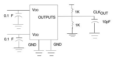
Test Circuit for t8, Output Slew Rate On -1H, -2H, and -5H Device
