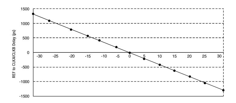
OUTPUT LOAD DIFFERENCE BETWEEN FBK PIN AND CLKA/CLKB PINS (pF)
