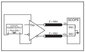
LVDS Output Load AC Test Circuit
