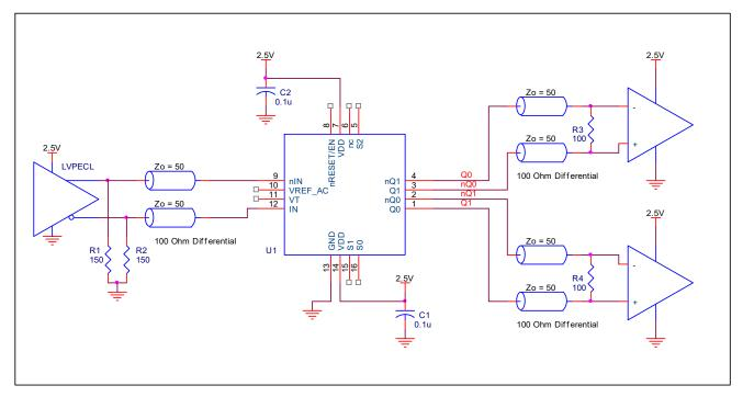
Figure 5. 8S89875I Schematic Example
