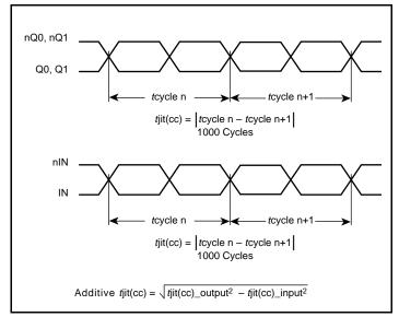
Additive Cycle-to-Cycle Jitter, RMS
