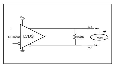
**Differential Output Voltage Setup**
