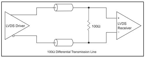
Figure 4. Typical LVDS Driver Termination
