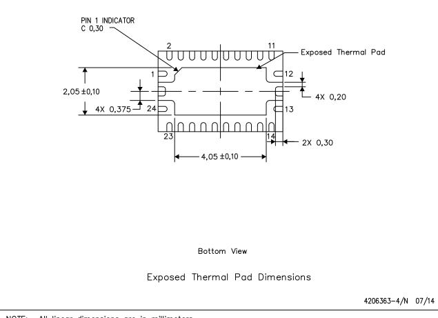
NOTE: All linear dimensions are in millimeters
